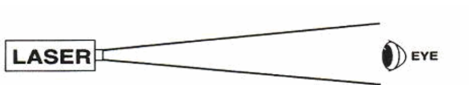
Figure 4 - Intrabeam viewing of direct (primary) beam. This type of viewing is most hazardous.
